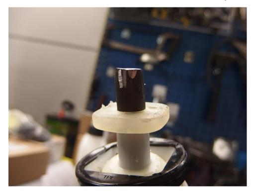
Cut the lower part of the gear shaft.
