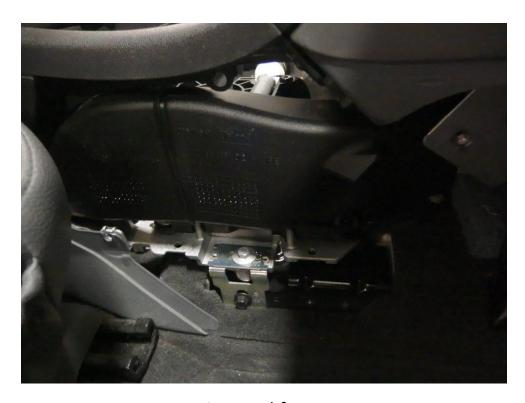
Remove AC tunnel for easy access.
