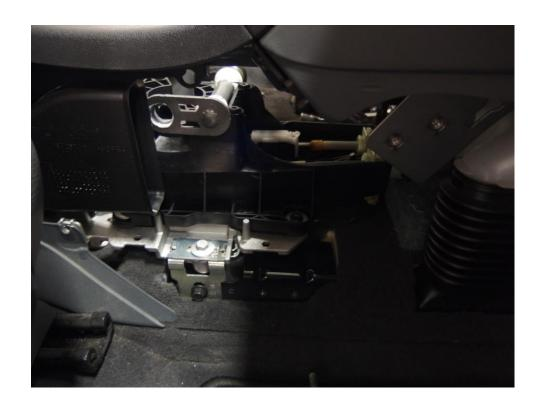
Remove four screws holding gear lever in place.
