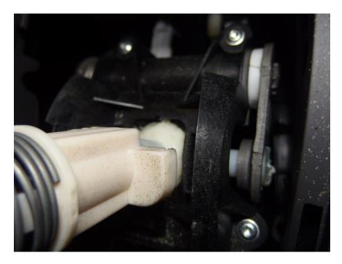
Remove 4 screws holding gear lever in position.
